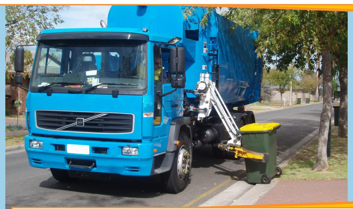
A truck picks up the bin and tips the recycling into the truck.
